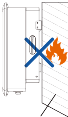
Wall material is flammable
